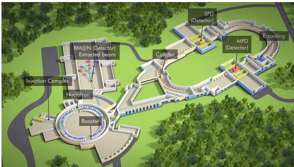
(a) Schematic view of the Nuclotron/NICA complex and the position of the BM@N setup.
