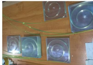
(c) Scintillator plates with WLS fiber in spiral grooves.
