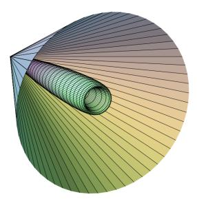
1.The angular distribution of the radiation is modified – the surrounding "funnel" appeared. The radiation is confined within the angle  $\theta_0$ :
