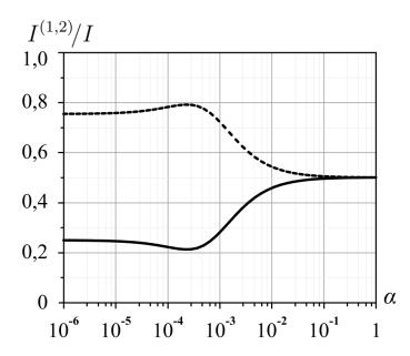
Linear polarization components of the radiation power depending on matter density parameter  $\alpha$ :  $I^{(1)}/I$  (solid line),  $I^{(2)}/I$  (dashed line); p=1 keV, m=1 eV
