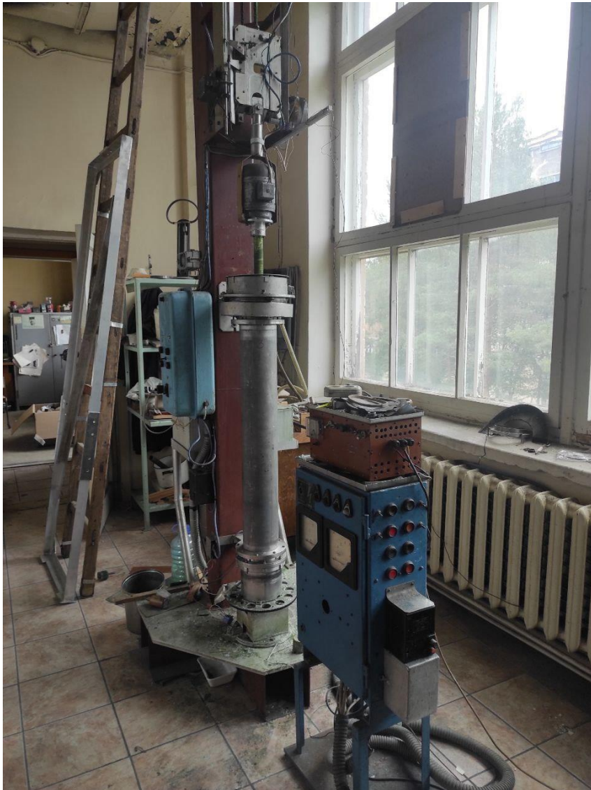
Pipe final polishing machine
