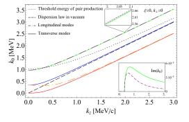
The figure shows the laws of dispersion of plasmon-polariton modes for a single unpolarized electron in the electron rest frame. The law of dispersion in vacuum and the threshold for the formation of an electron-positron pair are also shown. The energies of plasmon polaritons exceeding the pair formation threshold have positive imaginary parts shown in the inset.
