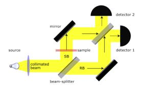
The scheme of the Mach—Zehnder interferometer. A solitary electron is supposed to be placed as a sample in one of the arms of the interferometer. For this experiment, it is necessary to calculate the phase shift of an electromagnetic wave when passing through an electron wave packet.
