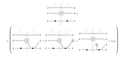
Diagrams illustrating the contribution to the inclusive probability of photon detection in stimulated radiation by a single electron in the presence of an external electromagnetic field.
