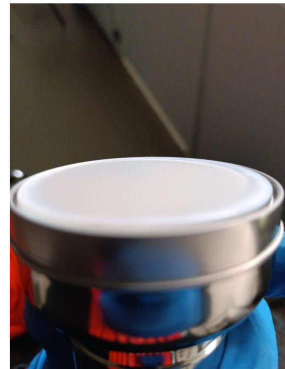
The same PMT coated with TPB
