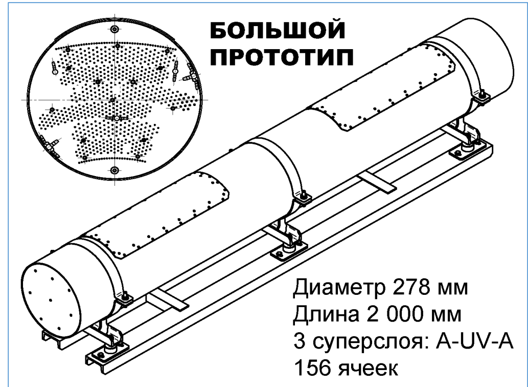
Large prototype (under construction) – 156 cells
