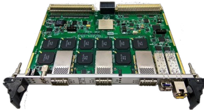
72-channel time-to-digital converter TDC72VHL v4 with CXP input connector.
