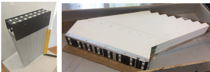
Top – evolution of ECal module shape from the center to the edge of MPD, bottom - modules of different types.
