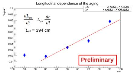
We can not separate aging of the scintillator and of the conversion efficiency of the WLS fiber. But we observe a hint of some decrease in its attenuation length. The increase of aging effect with the distance from SiPM gives an estimation of WLS attenuation length shortening  $-dL_{att}/dt = 0.37 \pm 0.07 \text{(stat.)} \%/\text{year}$
