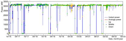
Reactor power measurements with  $\tilde{\nu_e}$ . Normalization from a short period at the beginning of data taking.
