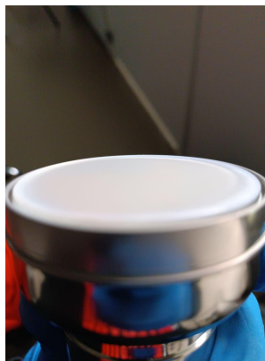
RED-100 PMT coated with TPB
