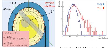
TFC algorithm gives efficiency of 92.4  $\pm$  4% for the price of 36 % live time loss
