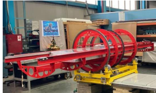
TOF installation bench in LHEP
