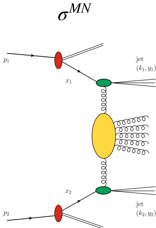
MN jet pair is a pair of jets with  $p_T$  above  $p_{T\text{min}}$  most separated in rapidity  $\Delta y = |y_1 - y_2|$
