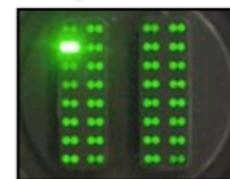
Scintillator cell with looped WLS Fiber.
