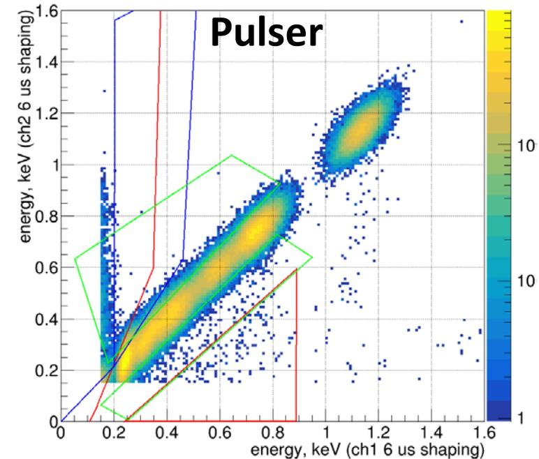
Efficiency measured with pulse generator
