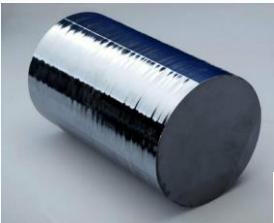
Silicon cryodetectors ( $T=10-50 \text{ mK}$ )
