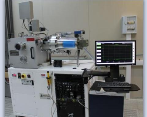
A photograph of an electron beam deposition system. It includes a large white vacuum chamber with a blue bellows, a computer monitor displaying a waveform, and various control panels and cables. |
