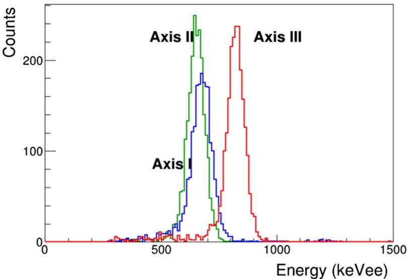
Energy spectra of 4.63 MeV  $\alpha$  particles impinging along the three axes of the crystal. The crystal was irradiated in the directions along the crystal axes I (blue on-line), II (green on-line), and III (red on-line), respectively
