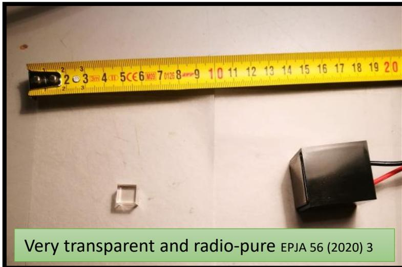
$\text{ZnWO}_4$  crystal = 10 x 10 x 10 mm<sup>3</sup> (detector of reduced dimensions to investigate neutron single-scattering)
