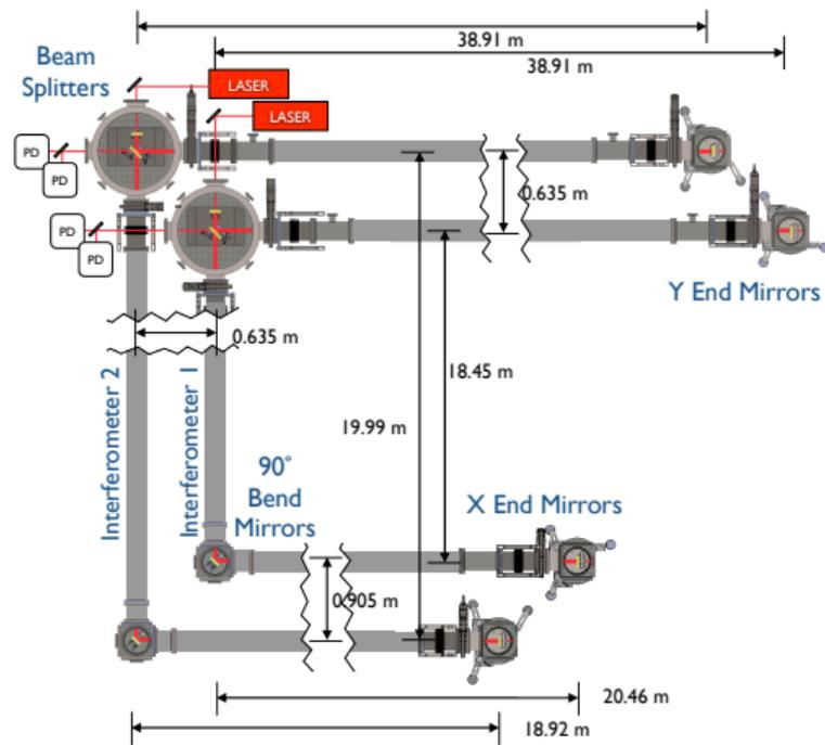
Bend mirror added. Unmodified: optics, electronics, control system, and data acquisition chain.
