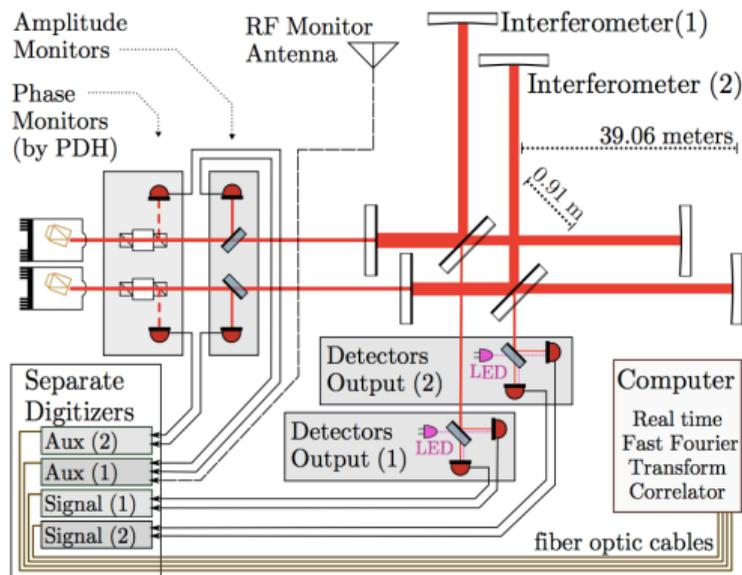
**Four RF environmental channels are cross-correlated with the interferometer output channels (8x8 correlation matrix)**
