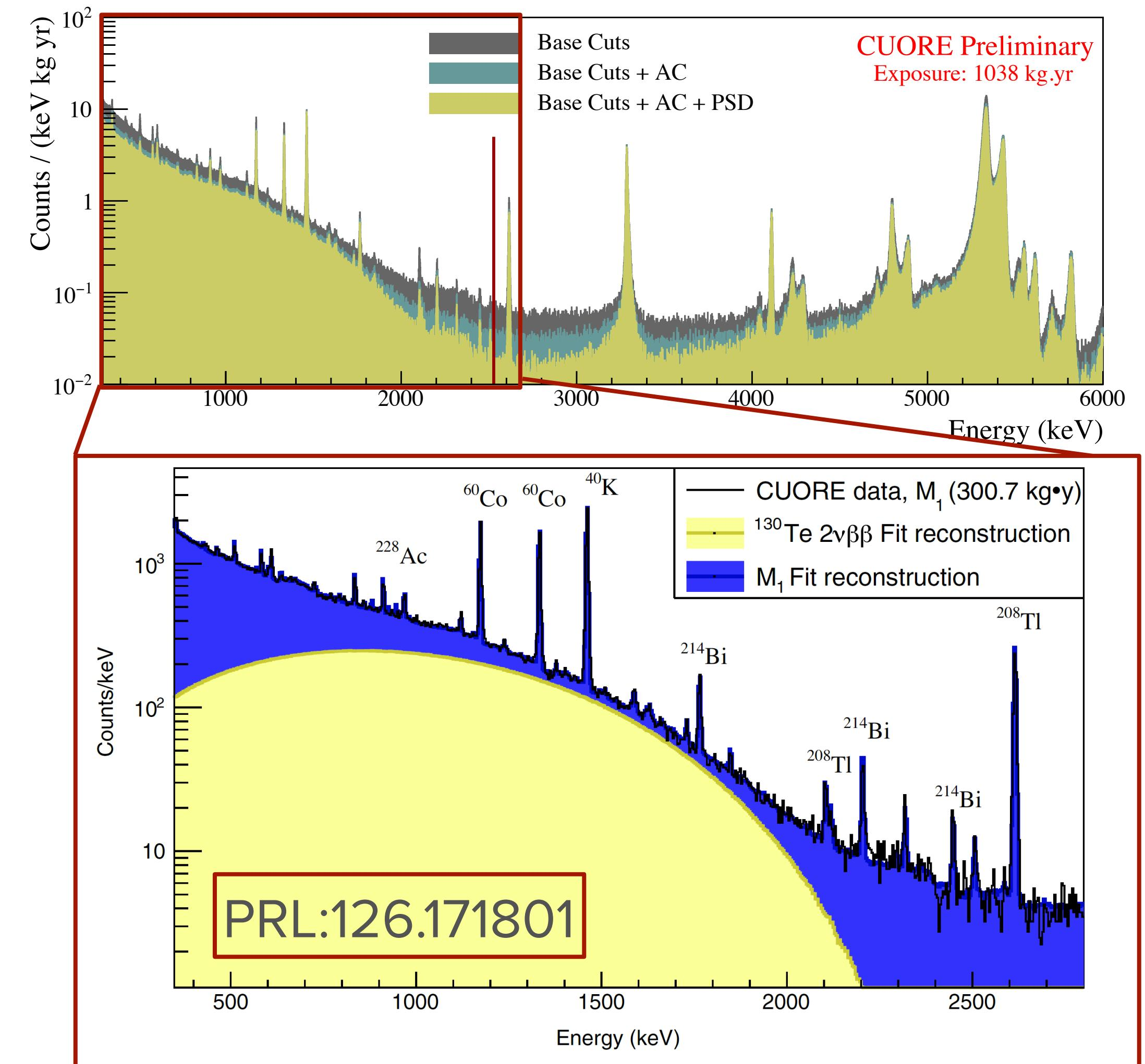
$$T^{2\nu} \frac{1}{2} ({}^{130}\text{Te}) = 7.71 + 0.08 \text{ (stat)} + 0.12 \text{ (syst)} - 0.06 \text{ (stat)} - 0.15 \text{ (syst)} \times 10^{20} \text{ yr}$$
