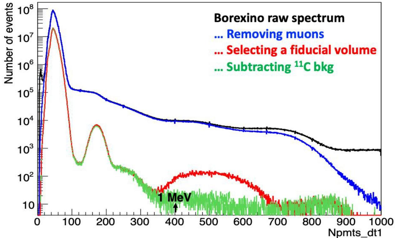
$^{11}\text{C}$  can be tagged and removed exploiting the space and time correlation between the parent muon the spallation neutron(s) and the  $^{11}\text{C}$   $\beta^+$  decay
