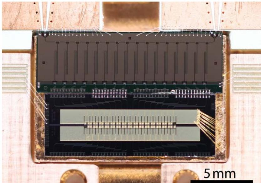
ECHo-100k baseline: large arrays of metallic magnetic calorimeters
