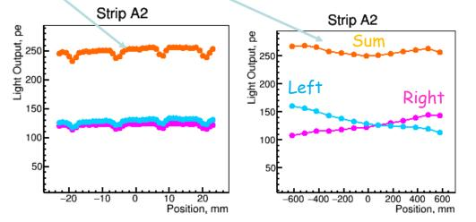
Longitudinal nonuniformity can be further corrected More work on SiPM-WLS fiber connection is needed
