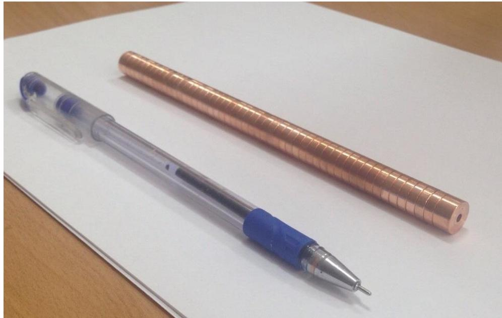
First prototype at BINP, frequency of 96 GHz
