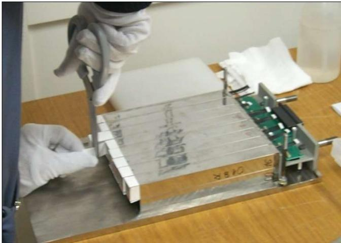
Crystals are packed mechanically into groups of 2x8, referred to as Strip units
