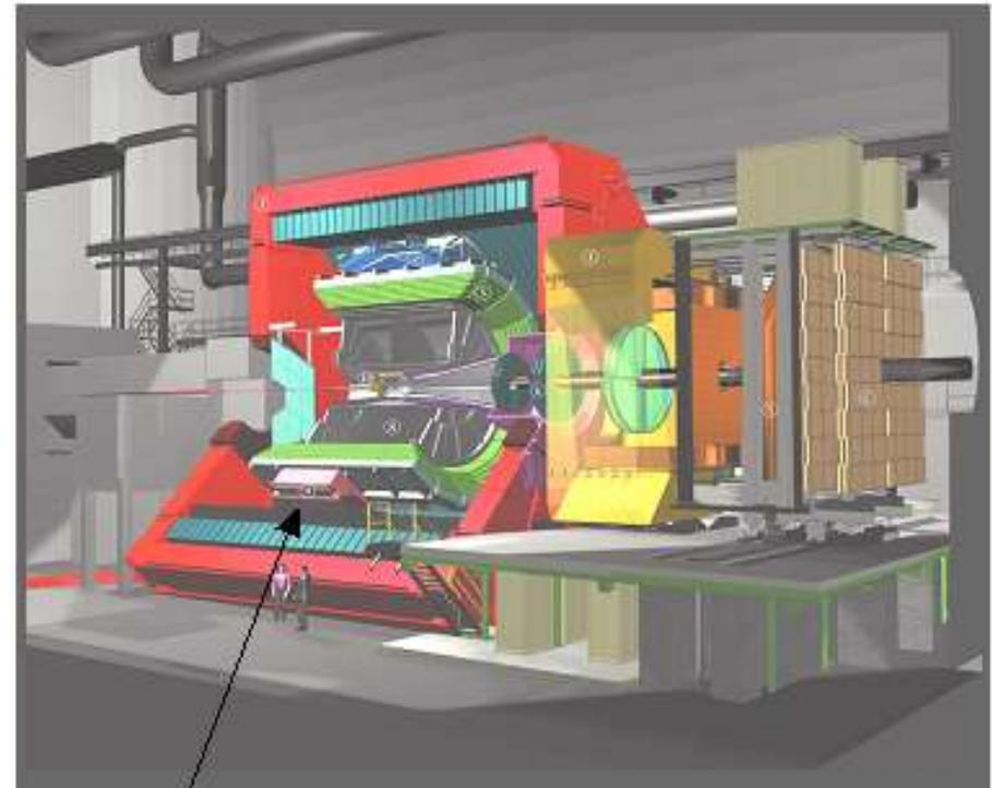
**PHOS (PHOTon Spectrometer) is a high resolution electromagnetic calorimeter consisting of 17920 detection channels based on lead-tungstate crystals(PWO).**
