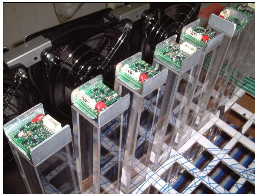
The detection channels with installed APD-photodiodes and preamplifier boards
